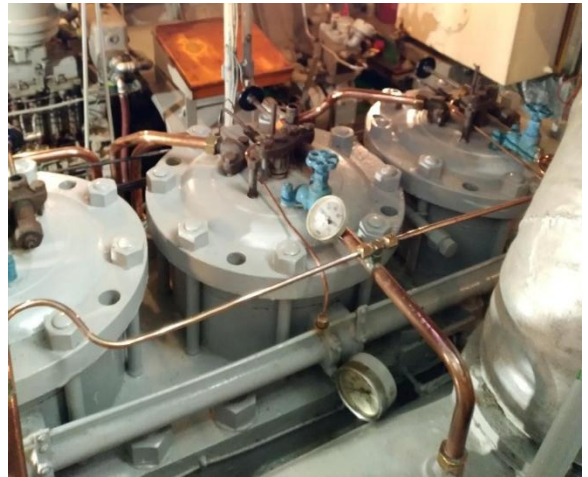
The huge three cylinder two-stroke diesel motor with its magnificently maintained brass work.
